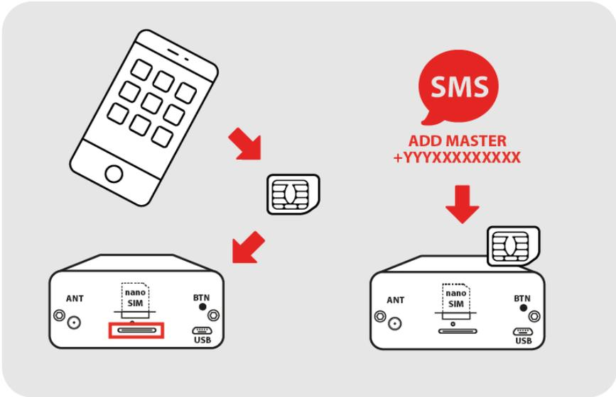
Insert the SIM card back into GSM KEY and send an SMS to its number in this form
