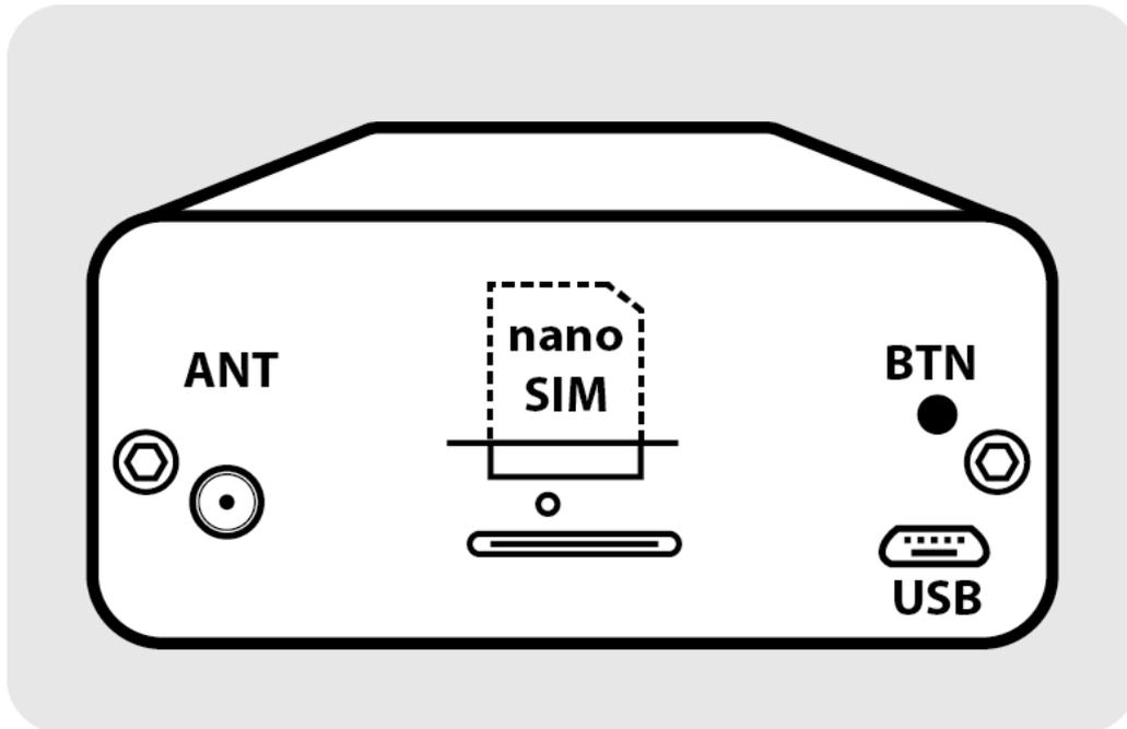
nano SIM: nanoSIM card insertion slot and blue LED signal
