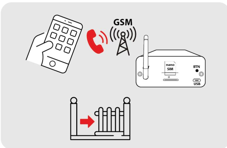
Your GSM KEY is now ready to use. To test that it is working, call the phone number of the SIM located in GSM KEY.
