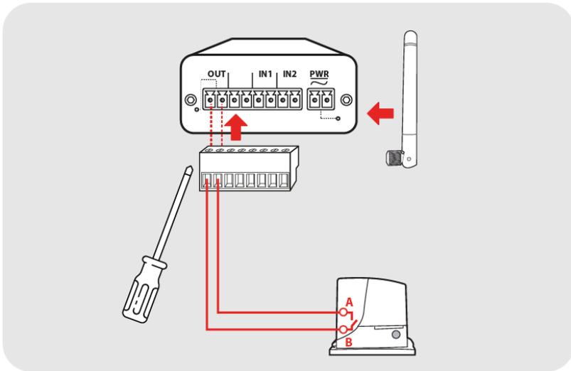
Connect the signal wire (minimum 2x 0.35 mm<sup>2</sup> Cu) to the OUT GSM KEY terminals and START terminals of your gate drive. Connect the antenna.
