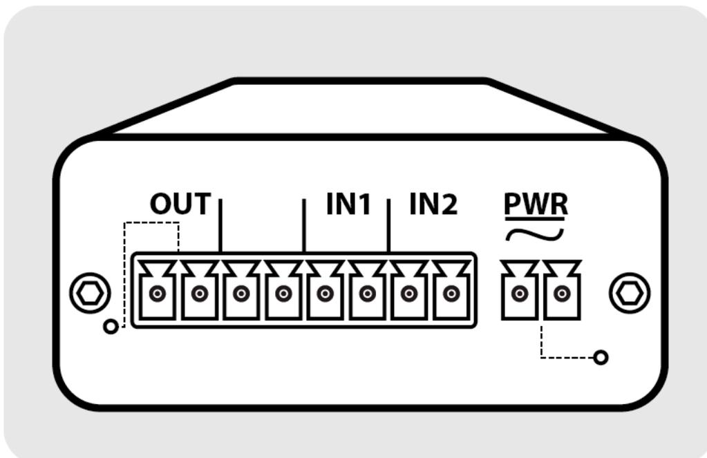
OUT: terminals for connecting relay-operated equipment (gate, door, barrier, boiler, etc.) with LED signal
